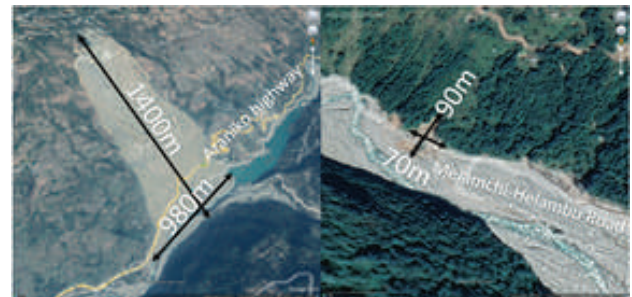
Figure 4 Landslide blockage locations at roadsides seen in Google Earth historical imagery.
