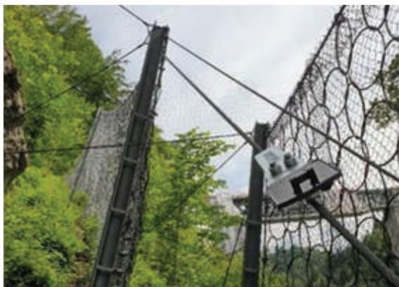
Figure 3: Example of an installed digital device called Geobrugg GUARD.
