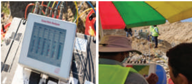
Figure 9: Cross hole Analyzer (KTFT Road Project)
