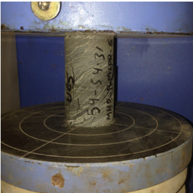
Figure 1: Rock fracturing after UCS testing
