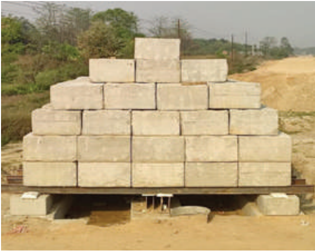
Figure 11: Static Load Test (Kent ledge Method)
